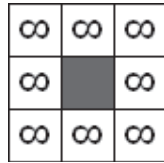
FIG. 3. Since the surrounding points currently have T values of infinity, an update at the center grid point will not yield useful information.
